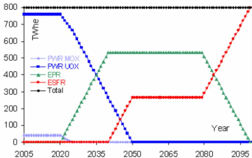
Figure 2: Assumed evolution of the electricity production, per reactor technology, for the Low Energy-Demand scenario of the CP-ESFR project. The above time schedule is an imposed input to the scenario.
