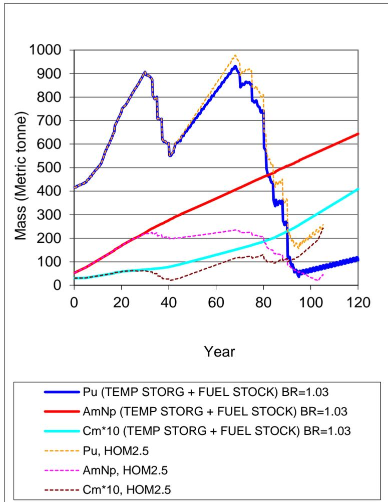
Figure 3: Material in Temporary Storage and Fuel Stock, both added. Cases: Reference (solid lines, BR=1.03) and 2.5%w MA homogeneous transmutation (dotted lines, BR=1.07).
